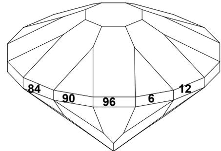
Figure 13, Placing the C2 facets
