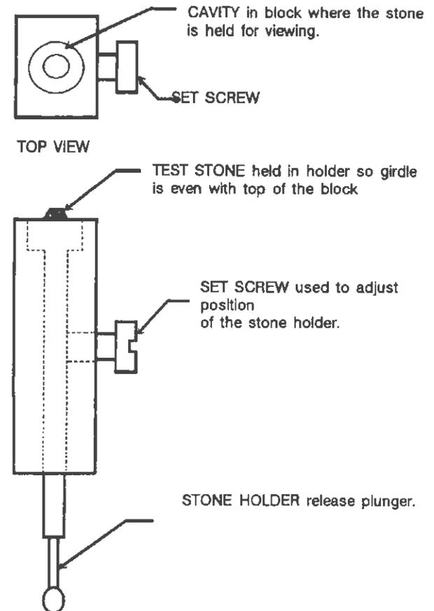
Figure 4 Features of Wolkonsky's modified stone holder which eliminates back reflections.
