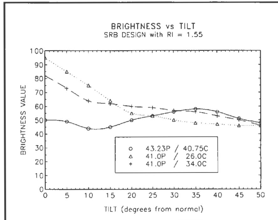
Figure 3 BRIGHTNESS vs TILT for selected SRB RI=1.55 designs
