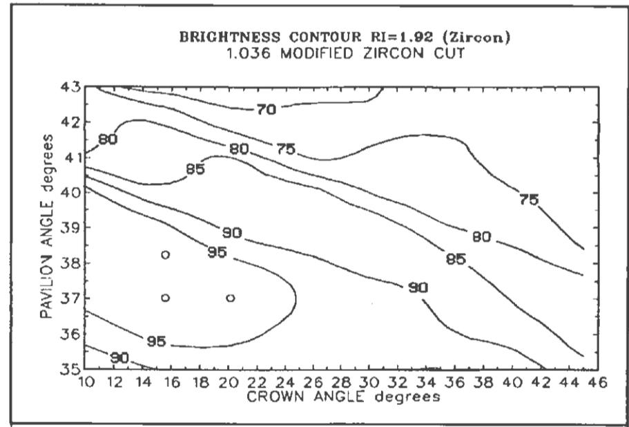
Figure 2 Brightness Contour plot for Zircon
