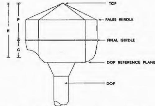
Figure 2 CAM Preform attached to a Dop
