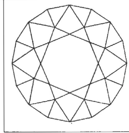
Figure 6 Brightness Plot for a 41P/24C Quartz 50% Table SRB. No dark areas visible. Brightness value 95
