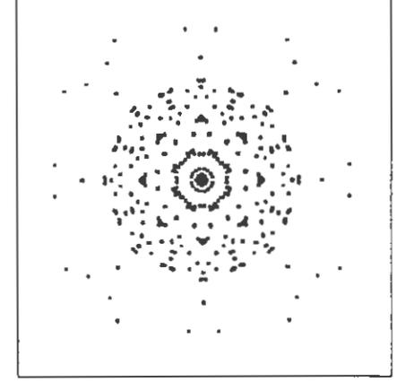
Figure 7 Reflection Plot for same design as Figure 6. Typical eight symmetry, light concentration points distributed in a definite pattern
