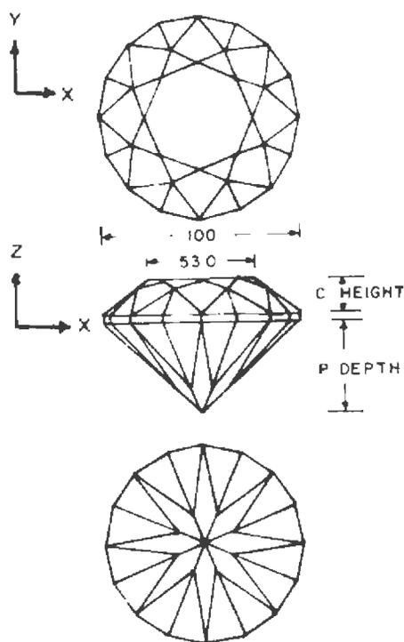
Figure 1 DIAGRAM OF STANDARD BRILLIANT
