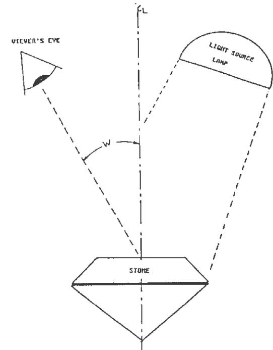
Figure 1 Relative position of observer, stone, and lighting lamp
